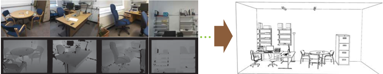
Figure 1: Automatic semantic modeling of an office scene. Left: input RGB-D images, right: reconstructed 3D scene.
