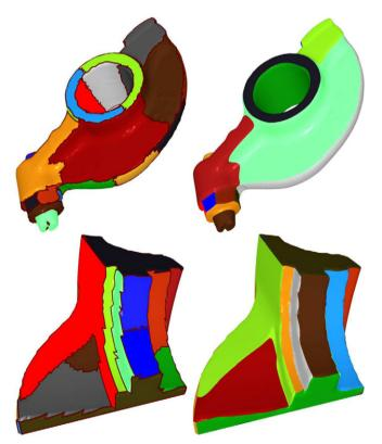
Fig. 8. Segmentation of engineering objects: rocker arm and fan disk. Left: initial segmentation with fine-scale seeding. Right: results after merging and smoothing.
