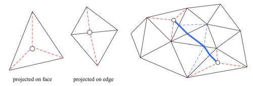
Fig. 2. Projection and local update of the input model. Left, center: mapping smoothed boundary points onto the surface. Right: mapping smoothed boundary paths onto the surface.
