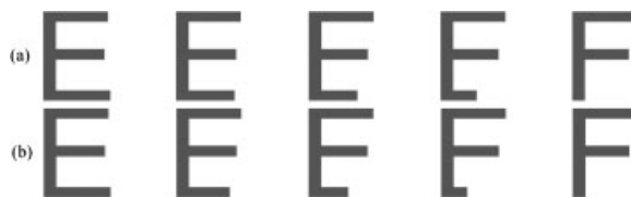
Figure 4. Morphing using (a) linear strain field interpolation, (b) modified strain field interpolation.
