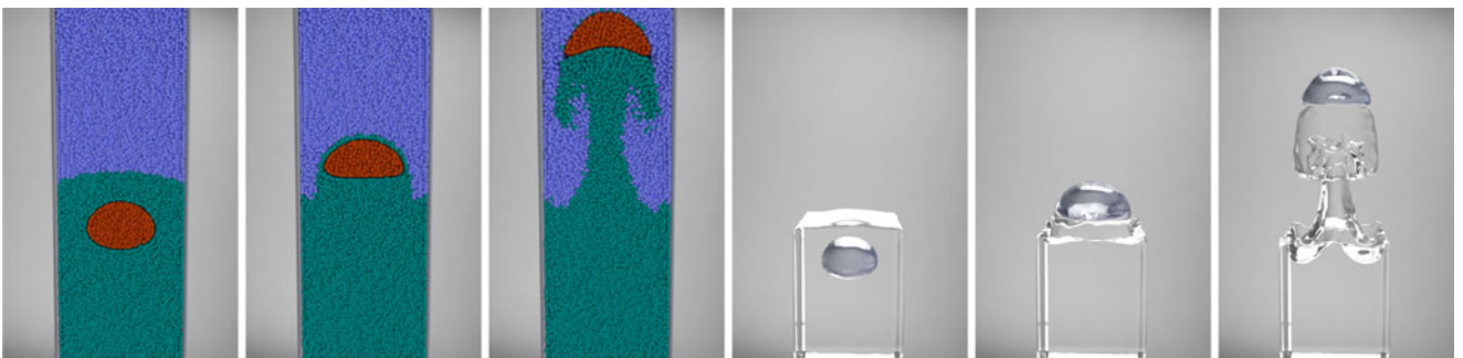
Fig. 17. Particle views, and rendered views, of a single bubble rising through a fluid-fluid interface. The rising bubble changes the interface shape by pulling the bottom fluid upward, and results in a mushroom-shaped column of the lower fluid being dragged upwards by the bubble.
