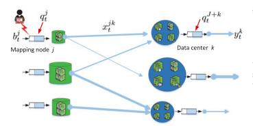
Fig. 1. A diagram of online network resource allocation. Per time t, mapping node j has an exogenous workload  $b_t^j$  plus that stored in the queue  $q_t^j$ , and schedules workload  $x_t^{jk}$  to data center k. Data center k serves an amount of workload  $y_t^k$  out of the assigned  $\sum_{j=1}^J x_t^{jk}$  as well as that stored in its queue  $q_t^{J+k}$ . The thickness of each edge is proportional to its capacity.
