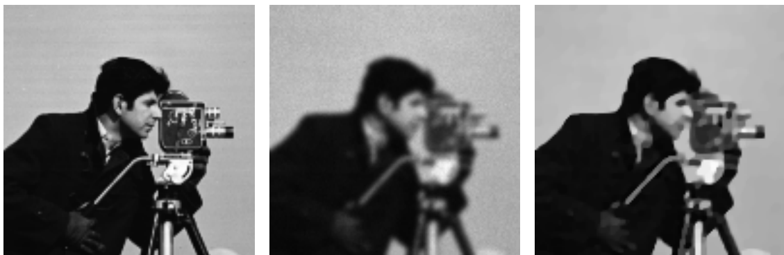
Figure 1: Left: Original image with values scaled to [0, 3000] so that the brightest pixels correspond to 3000 detected photons. Middle: Corrupted image blurred by a Gaussian kernel (standard deviation 1.3) and contaminated by Poisson noise. Right: Restoration result by the I -divergence constrained model (16) with total variation seminorm.
