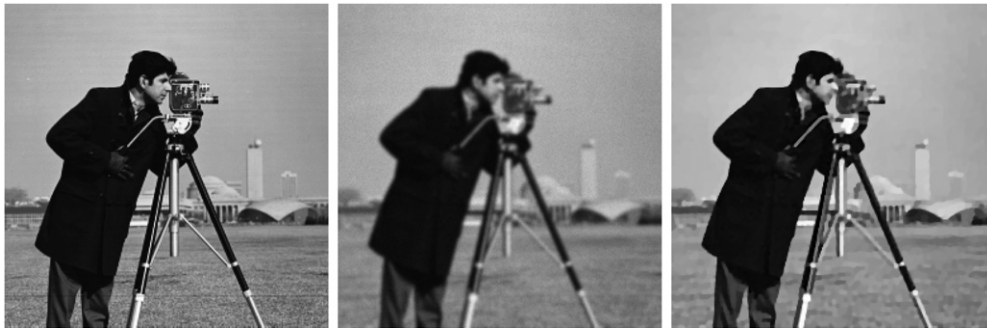
Figure 3. Result for the whole ‘cameraman’ image. Left: original image of size 256 \times 256 with values scaled to [0, 3000] . Middle: corrupted image. Right: restoration result by the l -divergence constrained model (16) with total variation seminorm.
