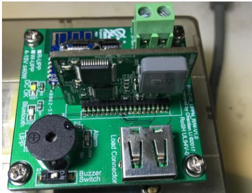
Image36-37 Prototype of UPP Low Voltage DC Power Adapter
