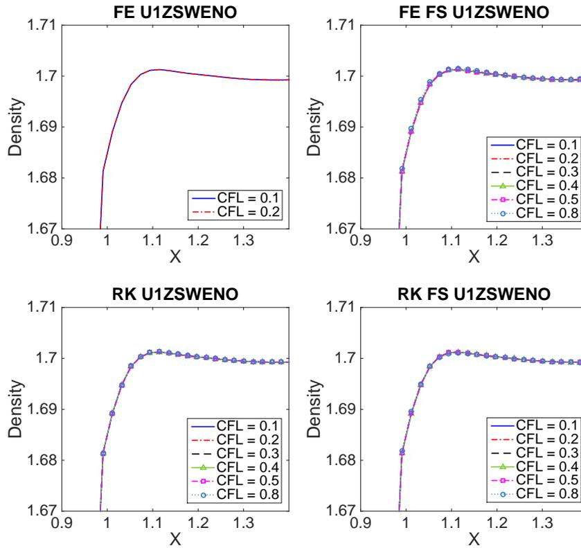
Figure 8: Example 6. Regular shock reflection. Zoomed density distribution near the impinging shock along the line  $y=0.5$  by four different iterative schemes with different CFL numbers. Top left: the FE Jacobi scheme; top right: the FE sweeping scheme; bottom left: the RK Jacobi scheme; bottom right: the RK sweeping scheme.
