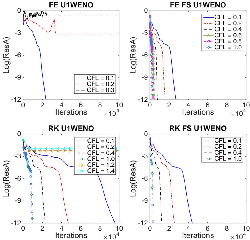
Figure 4: Example 5.  $135^\circ$  oblique shock of  $M_\infty=2$  problem. The evolution history of average residue along with iterations of four different iterative schemes with different CFL numbers. Top left: the FE Jacobi scheme; top right: the FE sweeping scheme; bottom left: the RK Jacobi scheme; bottom right: the RK sweeping scheme.
