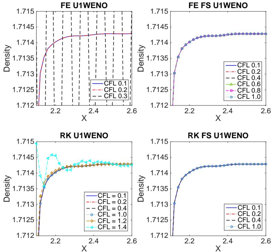
Figure 6: Example 5.  $135^\circ$  oblique shock of  $M_\infty=2$  problem. Zoomed density distribution (downstream) of the solutions along the line  $y=1$  by four different iterative schemes with different CFL numbers. Top left: the FE Jacobi scheme; top right: the FE sweeping scheme; bottom left: the RK Jacobi scheme; bottom right: the RK sweeping scheme.
