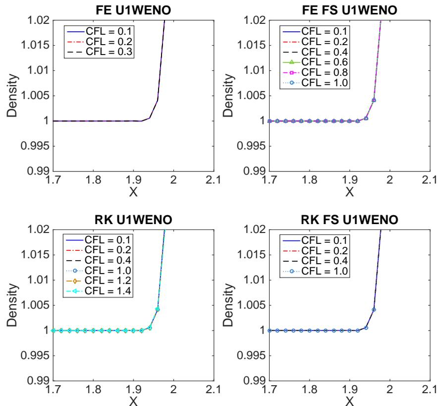
Figure 5: Example 5.  $135^\circ$  oblique shock of  $M_\infty = 2$  problem. Zoomed density distribution (upstream) of the solutions along the line  $y = 1$  by four different iterative schemes with different CFL numbers. Top left: the FE Jacobi scheme; top right: the FE sweeping scheme; bottom left: the RK Jacobi scheme; bottom right: the RK sweeping scheme.
