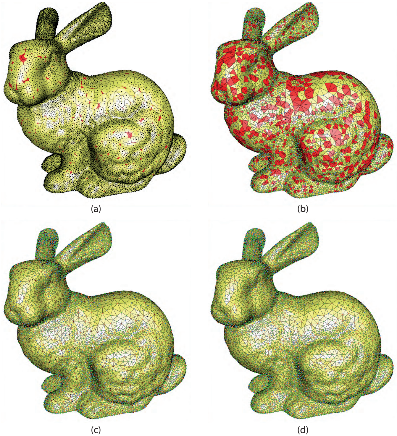
Fig. 1: Illustration of gap computation and valence optimization of the Bunny model. (a) The RPD and gaps on the surface, (b) remeshed triangles correspond to the non-maximal samples (red), (c) maximal sampling without optimization, (d) optimized remeshing. (The vertices with valence 5 (v5) are shown in blue, v6 green and v7 orange. Vertices with other valences are shown in dark.
