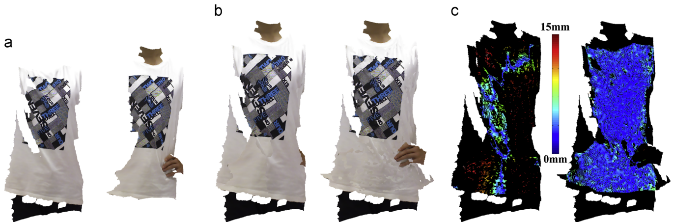
Fig. 15. Robustness in mid-scale registration. (a) The initial partial data before registration. Minor pose and cloth wrinkle changes cause difficulties especially if we try to use non-rigid alignment. (b) Overlap of the partial data before and after registration. (c) Euclidean distance changes for the closest vertex pairs before and after registration. Distances in the range 0–15 mm are rendered in pseudo-color. Vertices for which a closest vertex pair could not be found (largely for non-overlapping regions) are rendered as black, with a distance threshold of 15 mm.
