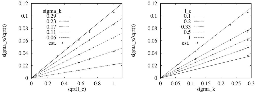
Figure 10. Influence of the standard deviation and correlation length of the Langmuir coefficient on the standard deviation of the shock position.
