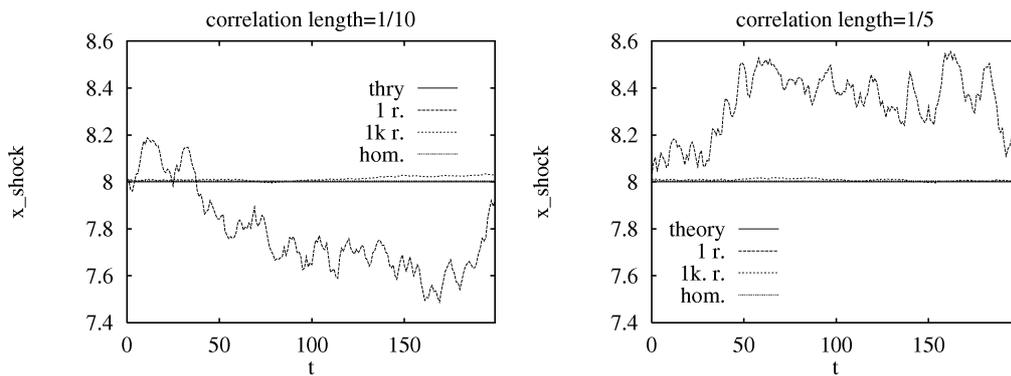
Figure 2. Position of the shock for correlation lengths 1/5 and 1/10.
