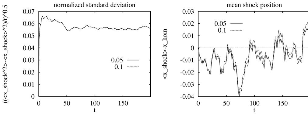
Figure 4. Influence of discretization on the mean and standard deviation of the shock position. Averages over 200 realizations.
