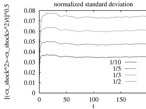
Figure 8. Influence of the correlation length of the Langmuir coefficient on the standard deviation of the shock position.
