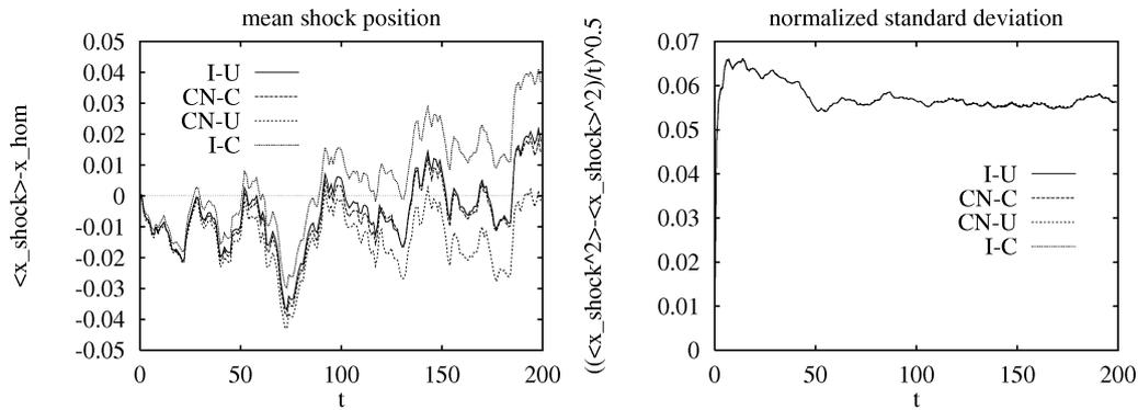
Figure 5. Comparison of different numerical schemes on the mean and normalized standard deviation of the shock position. Averages over 200 realizations. Coarse discretization.
