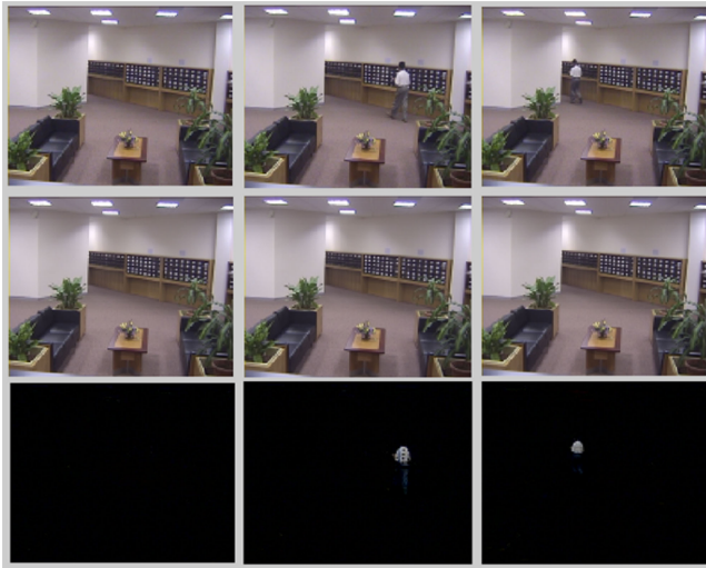
Fig. 3. Robust video recovery as robust tensor PCA. The first row are the 3 frames of the original video sequence. The second row are the recovered background, and the last row are the recovered foreground.
