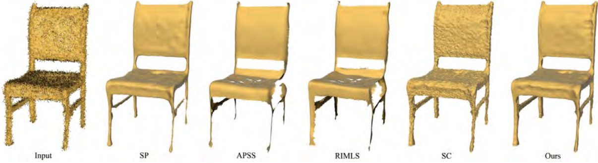
Figure 13: Various reconstruction results of the chair model. The point cloud is scanned by Kinect. The EAR algorithm is used to resample the noisy input into a clean point set with reliable normals.
