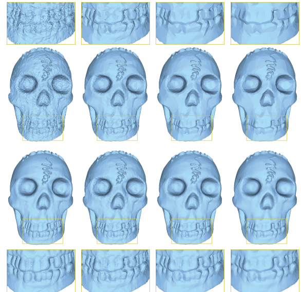
Figure 6: Skull model. From left to right: the second row shows the noisy input and then L_0 norm results by decreasing the fidelity parameter. The third row shows the original mesh and then our results by decreasing the fidelity parameter. The first and fourth rows show the local close-up views.
