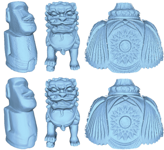
Figure 12: Denoising real scanned models: input models with noise (top) and denoised models (bottom).
