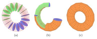
**Fig. 1.** A local bundle is a direct product of a disk and a circle, which is a solid torus. It can be represented by a prismatic mesh and further subdivided into a tetrahedral mesh, both with a regular structure that reflects the direct-product nature.
