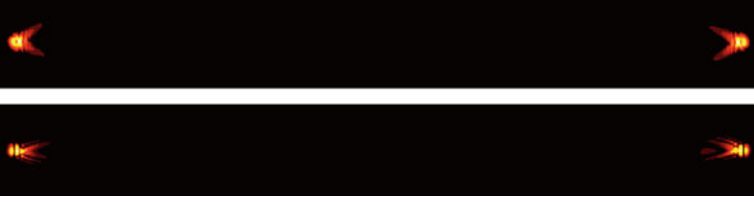
Fig. 9 Diffraction patterns for large deformations. Top: \beta = 0.005 Bottom: \beta = -0.01 . Here v = 0.1
