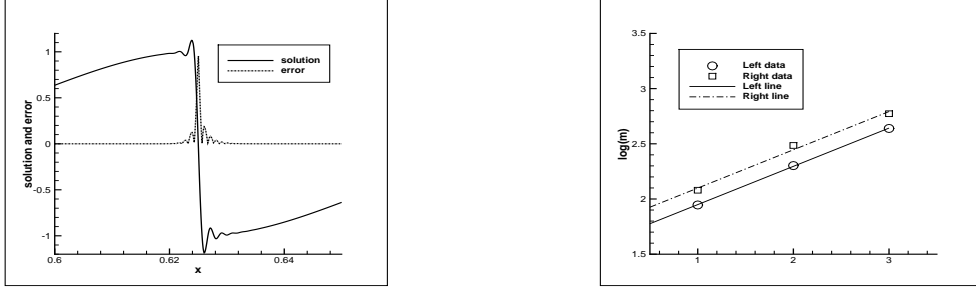
Figure 2: Example 3. Left: numerical solution and the error (in absolute value) for the coarsest mesh. Right: Dependence of the pollution region size and the mesh length.
