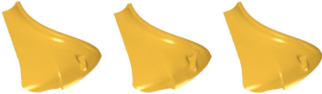
Fig. 10. Fitting a car part (left) by a cubic B-spline surface with 20 \times 30 control points and a FS parametrization (center); the result can be further improved with SDM (right).
