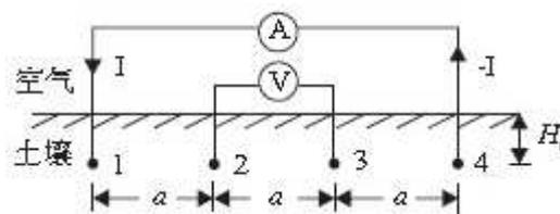
Figure 1 Routing of Venner Equidistant Four-pole Method
