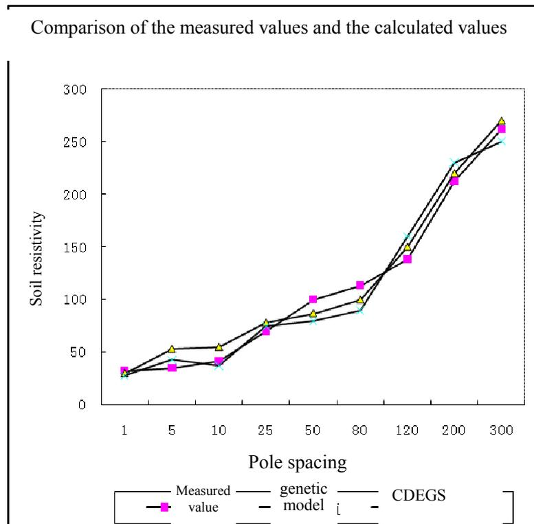
Table 2 Comparison between the measured and the calculated resistivity
