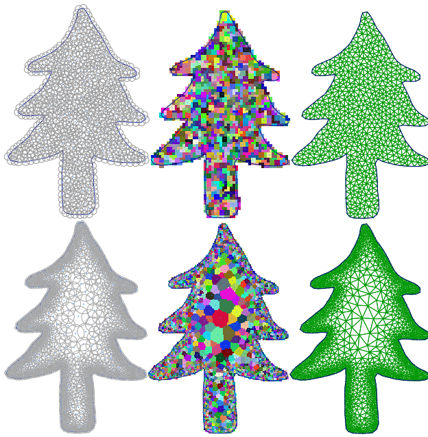
Fig. 1 Our algorithm can triangulate a uniform (top) and adaptive (bottom) Poisson-disk sampled point sets efficiently. From top to bottom, and left to right: uniform maximal Poisson-disk set, clustering result, and Delaunay triangulation; adaptively sampled Poisson-disk set, clustering result, and regular triangulation
