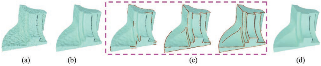
Fig. 1. Main phases of our approach: (a) the input noisy mesh model; (b) Phase I: denoising the model using DLRS (Section 4); (c) Phase II: recovering sharp features progressively based on \ell_1 -analysis (Section 5); (d) the final denoised result with recovered features.
