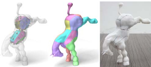
Figure 15: An assembled HORSE model (30cm tall; 18 laser-cut and 16 3D-printed parts) that can balance and stand on two legs.
