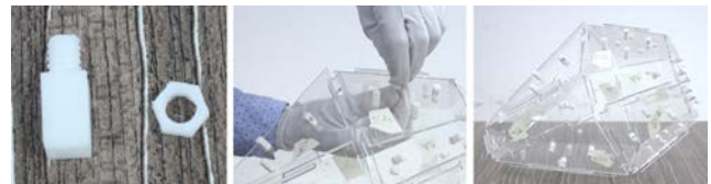
Figure 11: Install printed bolts and nuts in a laser-cut assembly.
