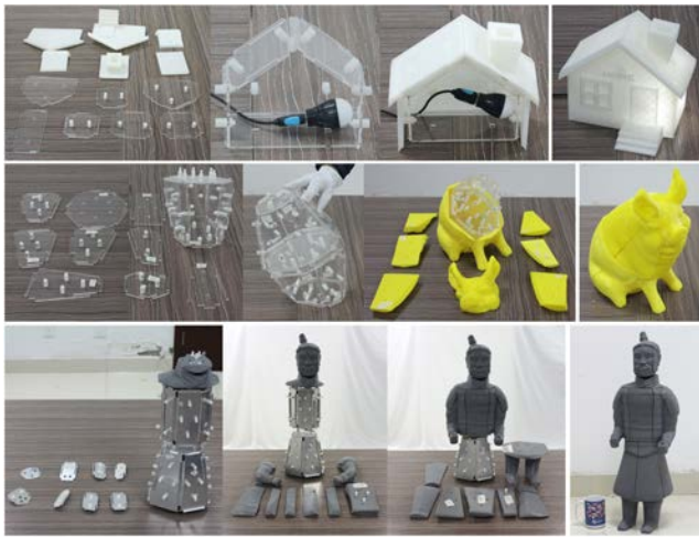
Figure 17: Physical fabricated assembly: HOUSE, GARDEN PIG, and TERRA COTTA WARRIOR models (from top to bottom). The diameters of 3D-printed bolts and nuts are 5mm and 8mm, resp.
