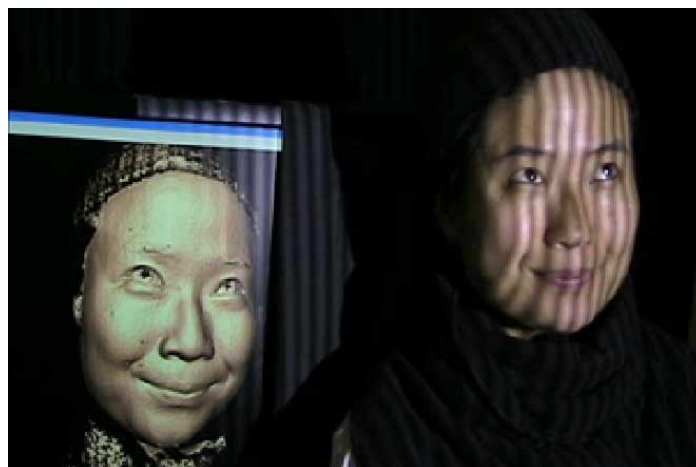
Fig. 6. (2.32MB) Real-time acquired, reconstructed, and displayed 3-D absolute coordinates at 30 fps.
