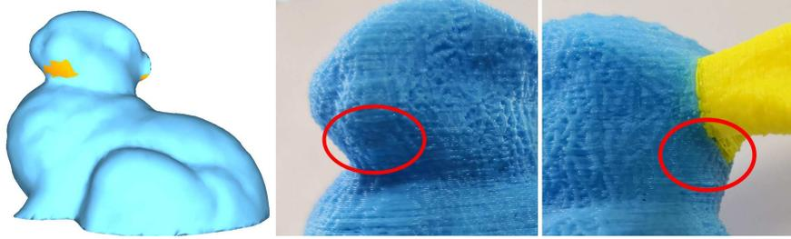
Figure 11: Surface quality of the printed bunny object using our printing system. Left: The regions with overlarge inclination angles are marked in yellow. Middle and right: the zoom-ins of the details in the two printed regions.
