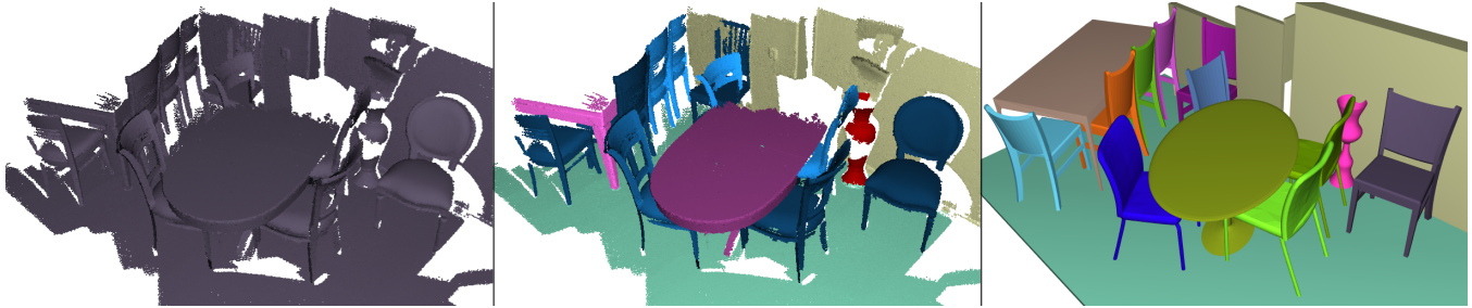
Figure 1: A raw scan of a highly cluttered indoor scene is given (left). Applying our search-classify method, we segment the scene into meaningful objects (middle: chairs (blue) and tables (purple)), followed by a template deform-to-fit reconstruction (right).
