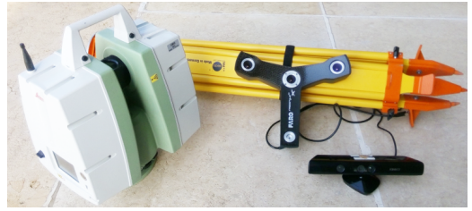
Figure 3: Three different devices used for capturing the input data to our system. From left to right, a Leica ScanStation C10 static laser scanner, a FARO Freestyle X hand-held scanner, and a Microsoft Kinect One depth camera.
