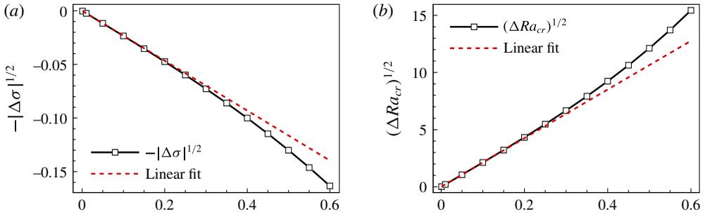
FIGURE 4. (Colour online) Variations of (a)  $-\lvert\Delta\sigma\rvert^{1/2}$  (for  $Ra = 2585.0187$ ) and of (b)  $(\Delta Ra_{cr})^{1/2}$  with  $\epsilon$  for  $A = 1$ . Linear fits of small- $\epsilon$  data (red dashed lines) are also depicted, indicating that  $-\lvert\Delta\sigma\rvert^{1/2}$  and  $(\Delta Ra_{cr})^{1/2}$  are proportional to  $\epsilon$  when  $\epsilon$  is small.
