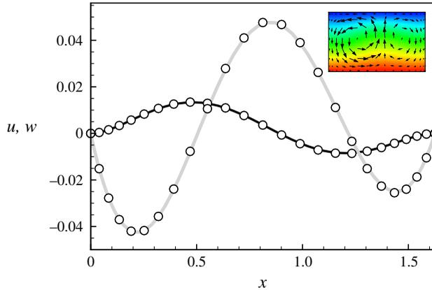
FIGURE 17. (Colour online) Profiles along the mid-plane  $z=0$  of the horizontal velocity component  $u$  (black line) and vertical component  $w$  (grey line) of the flow field (inset) constructed by weakly nonlinear analysis for  $(A, \epsilon, Ra) = (1.625, 0.2, 2490)$ . Results of DNS (circles) are also shown for comparison.
