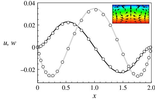
FIGURE 13. (Colour online) Profiles along the mid-plane  $z=0$  of the horizontal velocity component  $u$  (black line) and vertical component  $w$  (grey line) of the flow field (inset) constructed by weakly nonlinear analysis for  $(A, \epsilon, Ra) = (2, 0.6, 2300)$ . Results of DNS (circles) are also shown for comparison.
