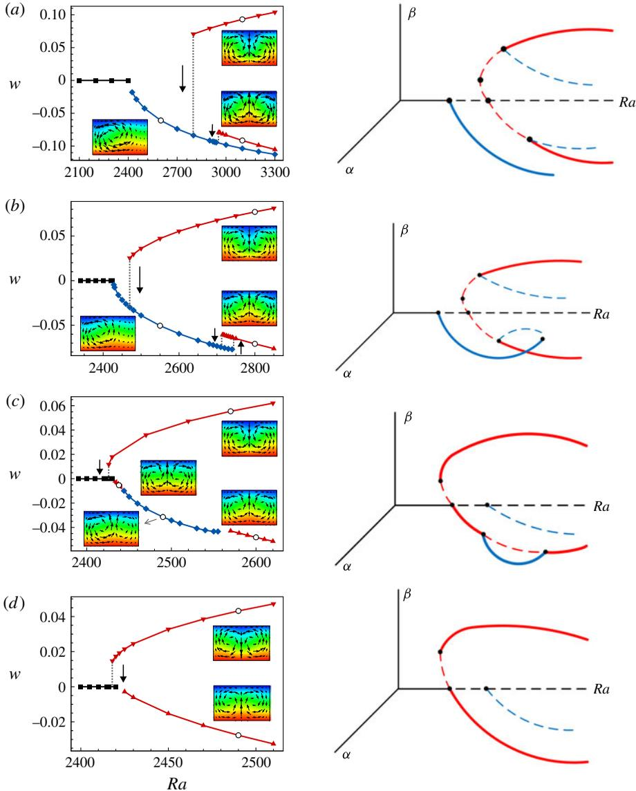
FIGURE 16. (Colour online) Bifurcation diagrams obtained by DNS (left column) and weakly nonlinear analysis (right column) for  $\epsilon = 0.2$  and (a)  $A = 1.58 < A_{cr}$ , (b)  $A = 1.61 < A_{cr}$ , (c)  $A = 1.625 > A_{cr}$  and (d)  $A = 1.63 > A_{cr}$ . In the bifurcation diagrams in the right column, stable (unstable) solutions are indicated by solid (dashed) lines. For clarification, two-roll and mixed-mode solutions are indicated by red and blue lines, respectively.
