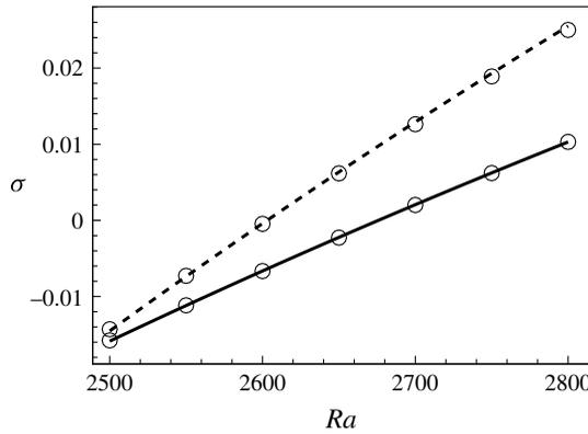
FIGURE 14. Growth rates of one-roll (solid line) and two-roll (dashed line) modes calculated by the weakly nonlinear analysis for  $(A, \epsilon) = (1.6, 0.6)$ . The results of the linear stability analysis (circles) are also shown for comparison.
