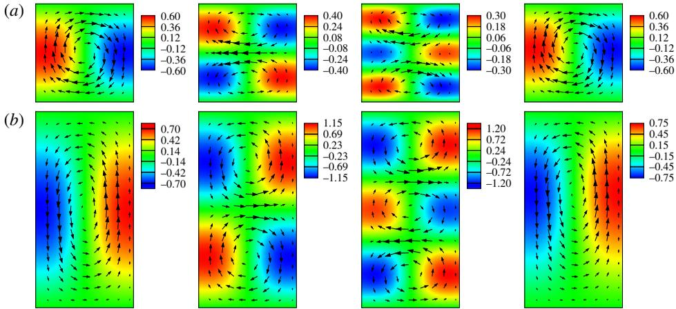
FIGURE 6. (Colour online) Velocity (arrows) and temperature (colour maps) distributions of  $\tilde{q}_0$ ,  $\tilde{q}_1$ ,  $\tilde{q}_2$  and  $\tilde{q}(\epsilon = 0.1)$  (from left to right) for (a)  $A = 1$  and (b)  $A = 0.5$ .
