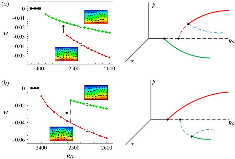
FIGURE 15. (Colour online) Bifurcation diagrams obtained by DNS (left column) and weakly nonlinear analysis (right column) within the OB approximation at (a)  $A = 1.62 < A_{cr,OB}$  and (b)  $A = 1.64 > A_{cr,OB}$ . In the bifurcation diagrams (right column), stable (unstable) solutions are indicated by solid (dashed) lines. For clarification, one-roll, two-roll and mixed-mode solutions are indicated by green, red and blue lines, respectively.
